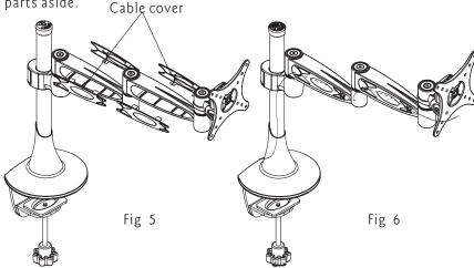
Route the cables along one side of the Inner Arm (nearest the wall plate). With cables in place, loosely secure the Inner Arm cable covers back in place. Next, route the cables along the opposite side of the Outer Arm. Be sure to leave slack in the cable where it transitions between two sides of the Arm Assembly. With cables in position, loosely secure the Outer Arm cable covers back in place.
